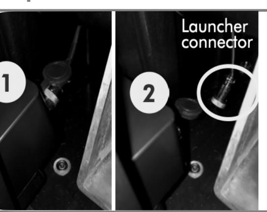
Disconnect the battery wire from the launcher connector.
