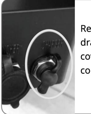
Remove battery drawer. Open cover of charger connector.
